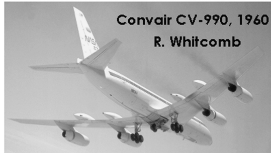
Fig. 40 Beginnings of transonic area ruling.
